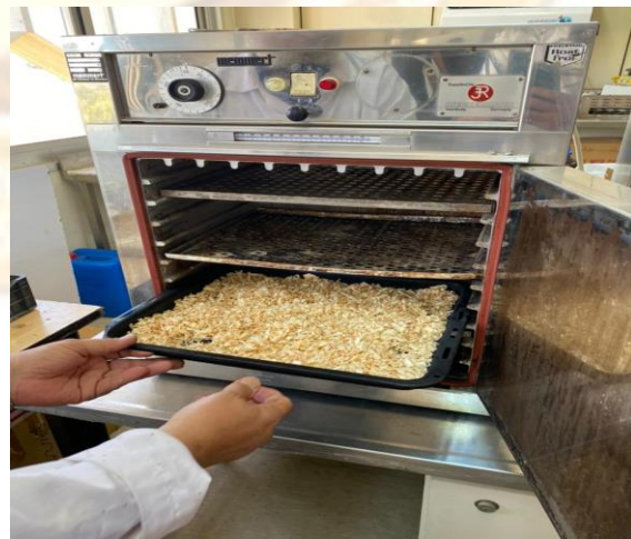
Figure 2.2: Dry the sawdust at temperature about 105\text{C}^{\circ}
