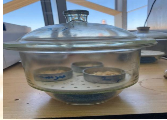
Figure 2.4 Measuring the moisture in the sawdust after drying
